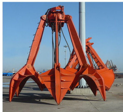
Figura 7: Cuchara de gajos ( Marine equipment supply )
